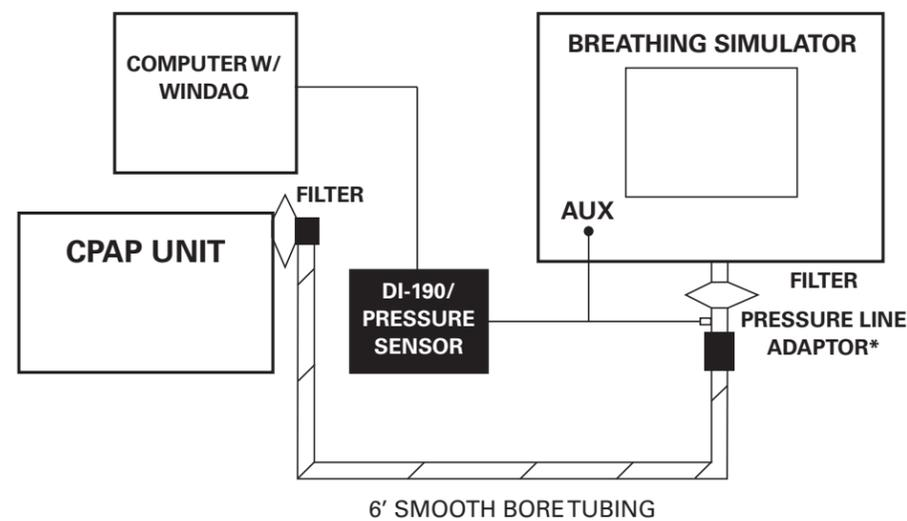
\*Pressure line adaptor is modified to allow passive exhalation, 25.5LPM @ 20cmH<sub>2</sub>O
