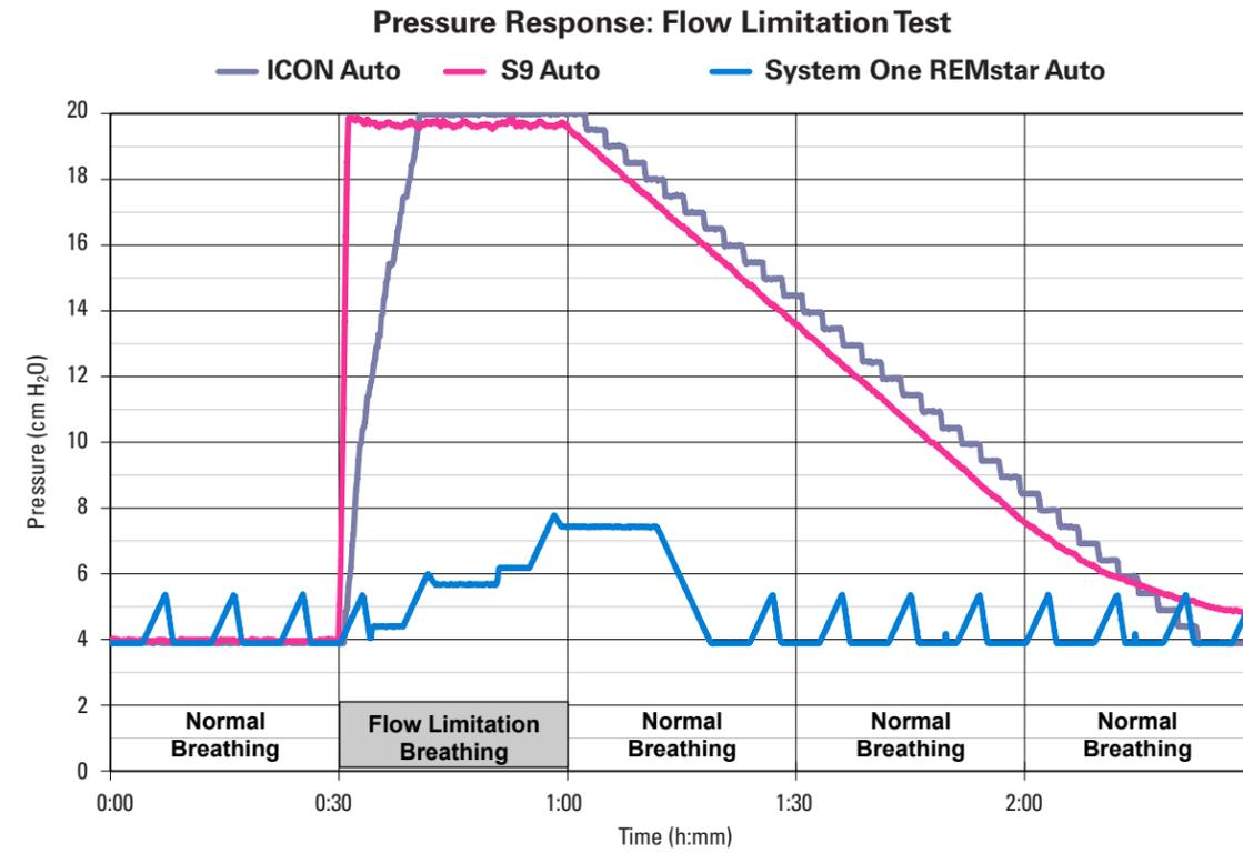
All devices exhibited pressure response to the change from Normal to Flow-Limited breathing. The ICON Auto unit showed a rapid pressure response, reaching a maximum of 20cmH<sub>2</sub>O within 15 minutes of the Flow Limitation pattern starting. The S9 AutoSet unit responded even more rapidly, reaching 20cmH<sub>2</sub>O within two minutes of the Flow Limitation pattern starting. Both units remained at 20cmH<sub>2</sub>O until
