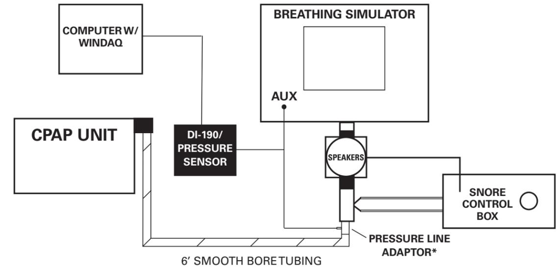
\*Pressure line adaptor is modified to allow passive exhalation, 25.5LPM @ 20cmH<sub>2</sub>O
